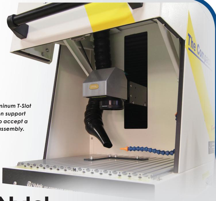
*All-aluminum T-Slot extrusion support ready to accept a fixture assembly.*
